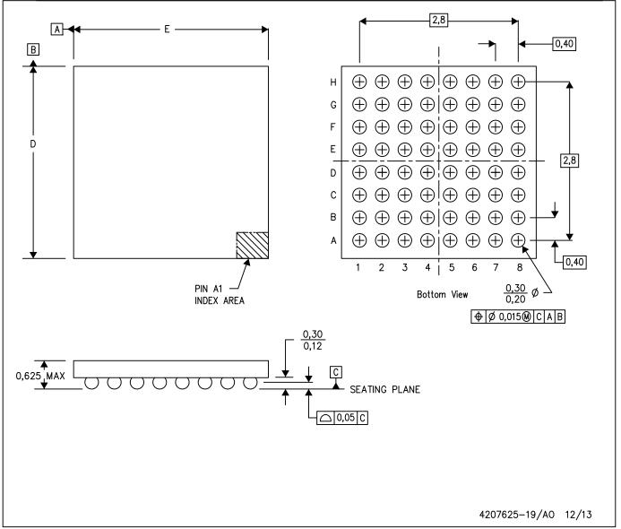
NOTES: A. All linear dimensions are in millimeters. Dimensioning and tolerancing per ASME Y14.5M-1994.
