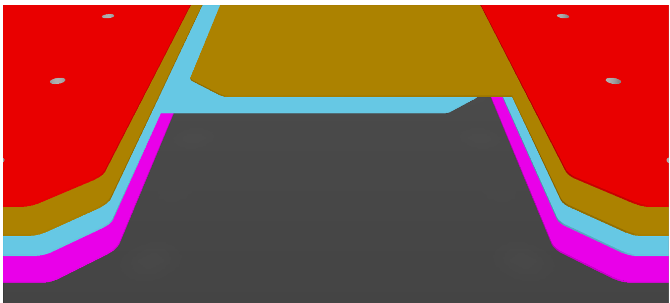
Figure 11. Triangle Corners Implemented to Enhance High-Voltage Performance
