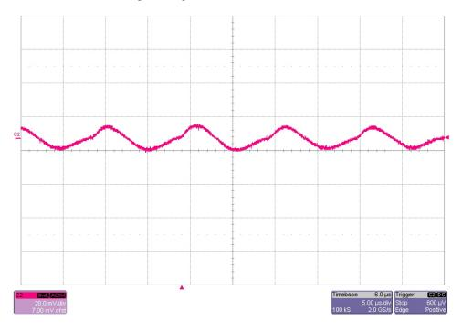
The 3.3V output ripple voltage is shown in the figure below. The image was taken with the 3.3V linear regulator loaded to 0.25A and the input voltage set to 12Vdc. (20mV/DIV, 5uS/DIV)
