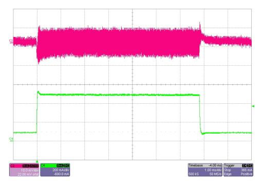
The photo below shows the 3.3V output voltage when the load current is stepped between 0.1A and 0.25A. Vin = 12Vdc. (20mV/DIV, 100mA/DIV, 500uS/DIV)
