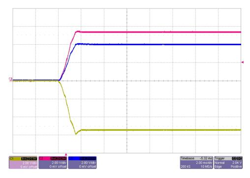
The photo below shows the flyback converter startup waveforms for the +4V, +5.5V and -5.75V output voltages after the application of 12Vdc in. The outputs were loaded to max loads. (2V/DIV, 2mS/DIV)
