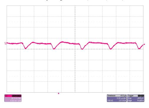
The 2.5V output ripple voltage is shown in the figure below. The image was taken with the 5V linear regulator loaded to 0.002A and the input voltage set to 12Vdc. (20mV/DIV, 5uS/DIV)
