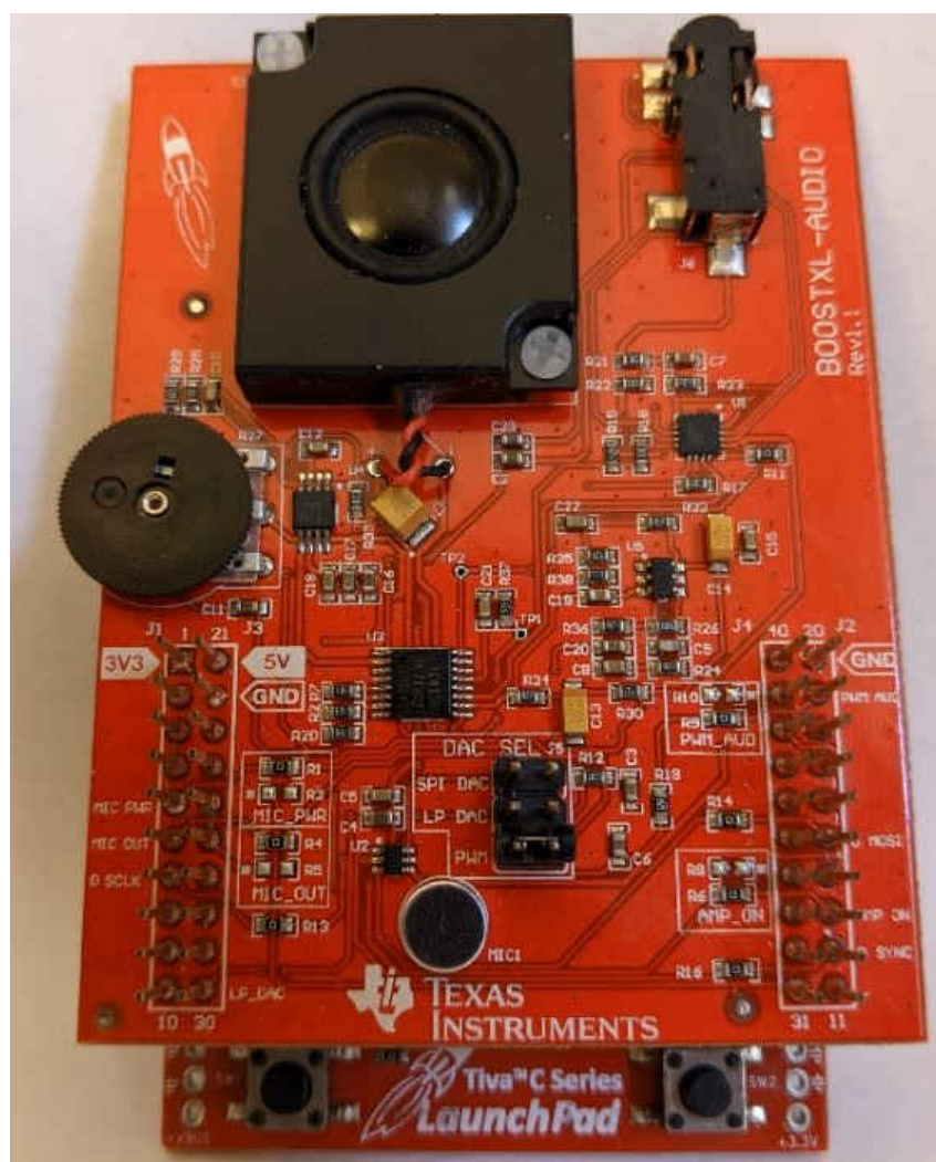
Figure 5-3. EK-TM4C123GXL LaunchPad With Audio BoosterPack
