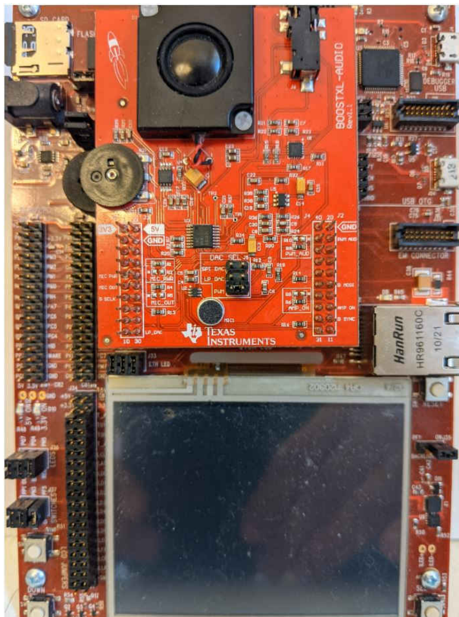
Figure 5-4. EK-TM4C129x Development Board With Audio BoosterPack
