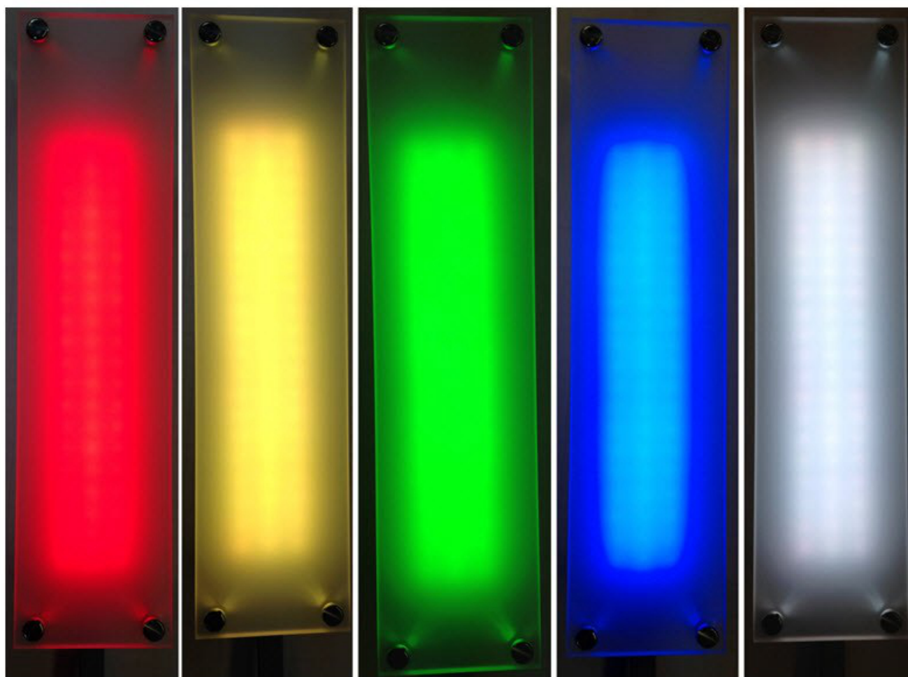
Figure 4. Five LED Segments behind Plexiglas Showing the Main Colors
