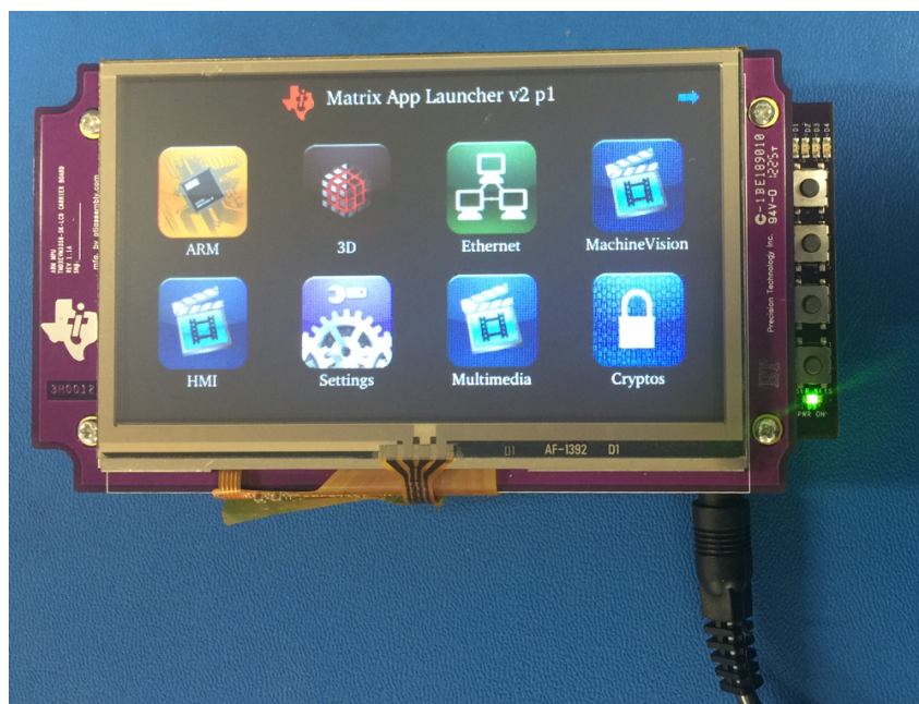
图 5. AM335x Starter Kit Setup (LCD Face Up)
